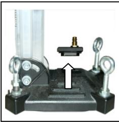
Remove the vacuum grip and the gasket of the base plate.
