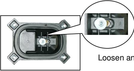
Loosen and remove the fastening nut.
