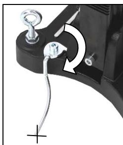
Mark the center of the hole to be drilled.
