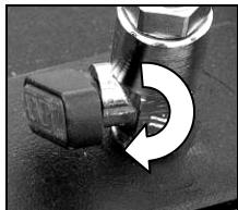
To unfasten the vacuum connection, close the valve. This opens a bleed valve through which the vacuum can escape. Thus the rig can be activated if necessary when the vacuum pump is running.
