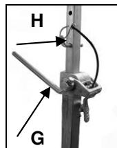
Position the drill rig. Position the quick action bracing unit as close as possible behind the support on the base of the rig. Fix the drill rig by turning the crank (G) clockwise. Secure in position by means of the appropriate bolt (H).
